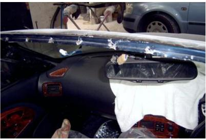
This should result in the subframe landing in your lap. The pictures below show the distinct lines of rust where the glue was applied:
