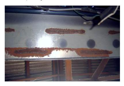
These need to be cleaned up to remove any loose rust, neutralised, undercoated and then the subframe needs to be welded back in place.
