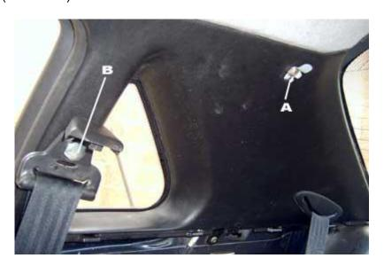
Step 8. Next, remove the 3 screws marked A in the illustration below.
