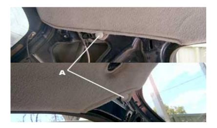
Step 15. The only thing holding in the lining now are the 2 clips shown below. To pop these pull the lining toward the front of the car. be careful, the lining is cardboard and will crease if you are not careful.
