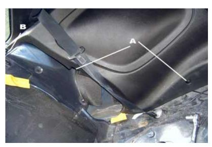
Step 5. There are 2 clips behind each side. The diagram below illustrates their location. Pop both clips (on each side) and remove lower panels by sliding toward the front of the car.
