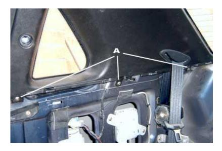
Step 9. This part has 3 clips on the back of it. The illustration below shows their location. Pop each of these and let the part dangle off the seat belt. You will not be able to completely remove it as the rear seat belt runs directly through it. Repeat process for the other side.
