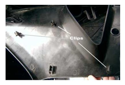
Step 10. The A pillar cover has 2 clips and a plastic lug that locates it on the pillar (shown below). Pop both clips and remove the pillar cover by pulling up towards roof. Repeat on other side.
