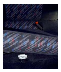
Step 3. Remove the upper portion of the rear seat. Use the 12mm socket to release the 2 bolts that are holding the bottom of the rear seat down. One of these is shown below.
