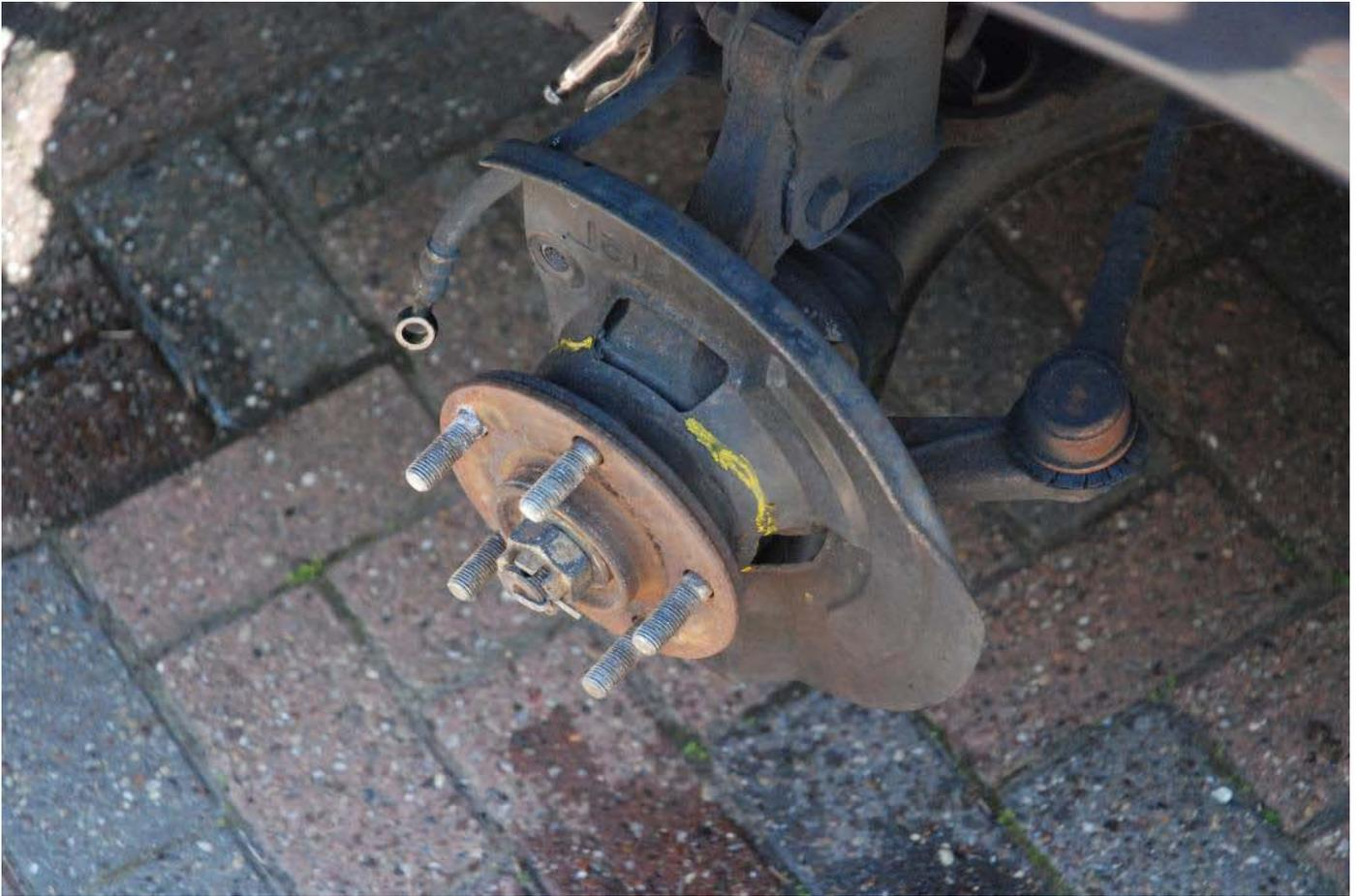
cut the back plate off by cutting the 4 joins to the hub, marked in the photo with a yellow line. clean up the rough edges if there are any.
