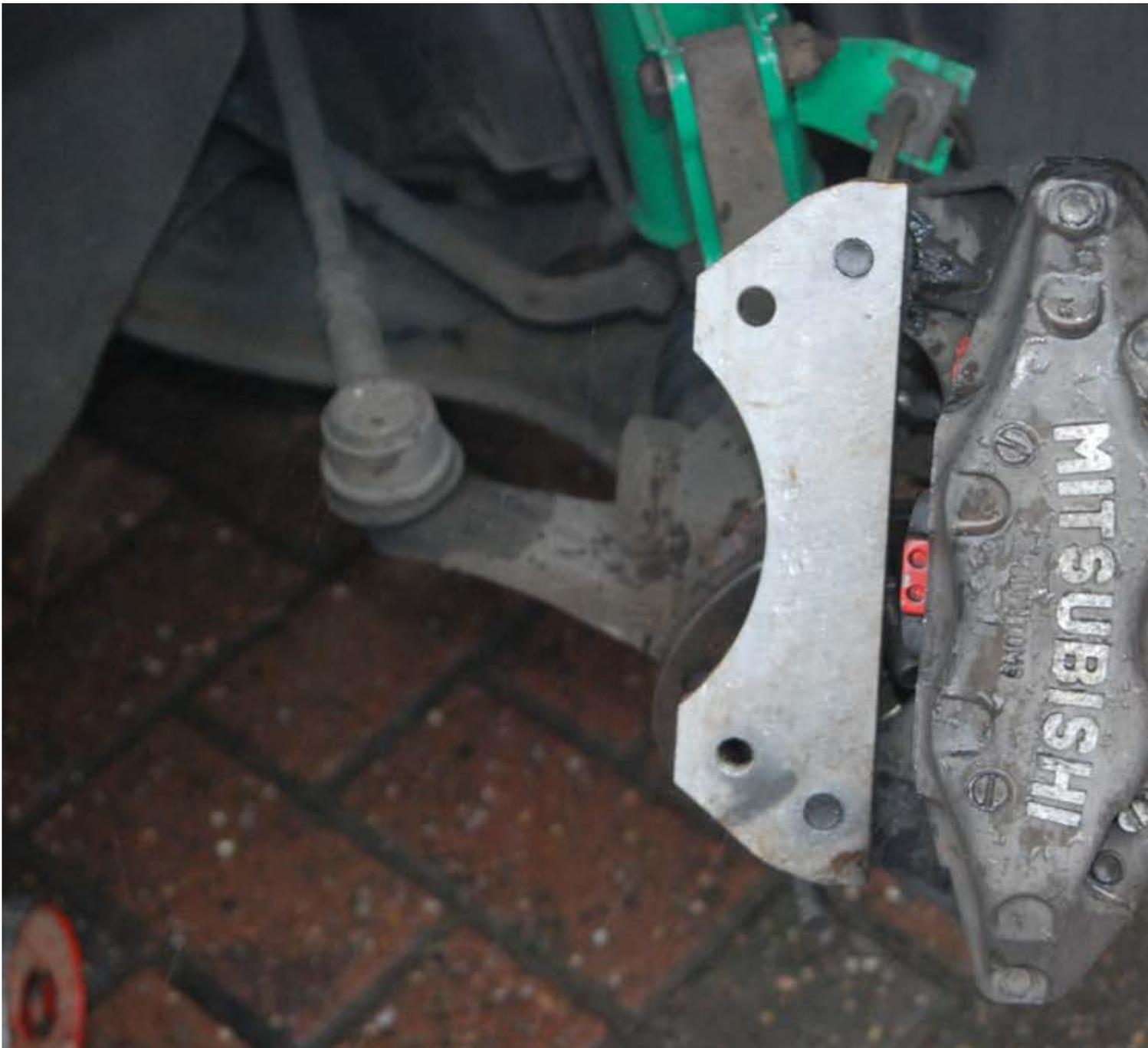
use the 17mm bolts that you removed from your old calliper to bolt the bracket to the hub. make sure all bolts are
